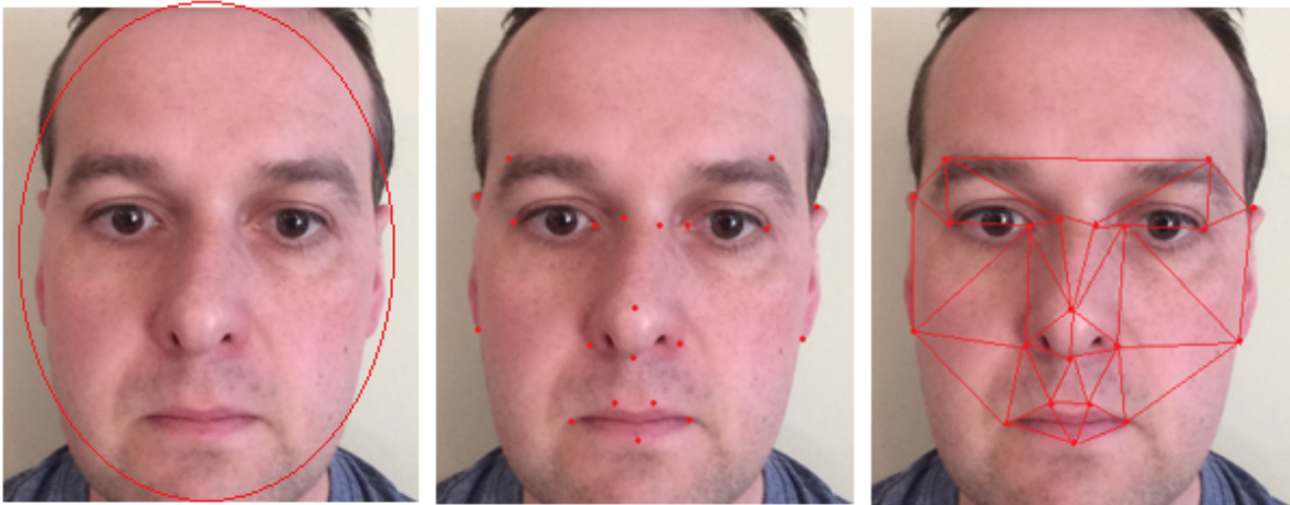
Figure 1 - First the face is found then specific points on the face located. Finally distances and geometry between points are calculated
