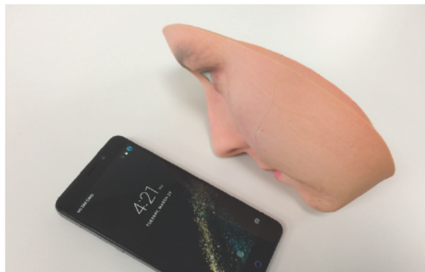
Figure 13 - Holding the mask in front of an Android camera for successful authentication bypass
