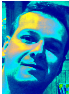
Figure 7 - Thermal imaging to detect heat and liveness might defend against image/mask spoof attacks
