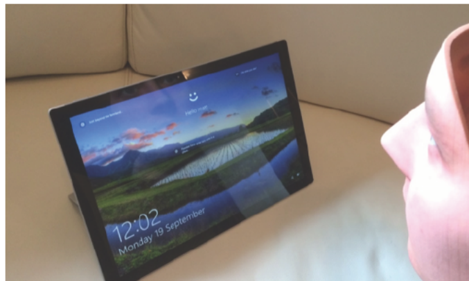
Figure 12 - Holding the mask in front of a Surface camera for successful authentication bypass (older Hello algorithm)
