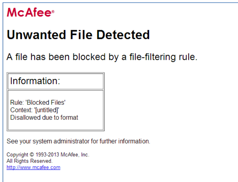
Figure 20 In this case the attachment in the message was replaced by a HTML file which ended up going back to the sender. This can lead to more policy and product disclosure.
